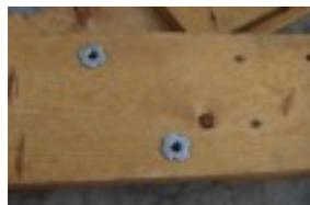
T-nuts on rail to mount cross bar
