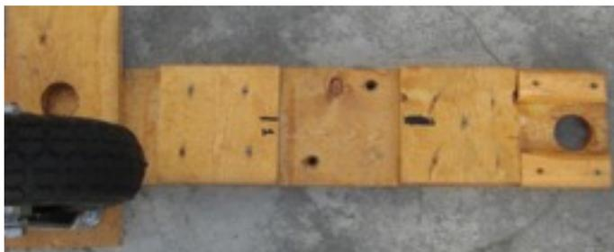
Image shows how cross bar mounts into rail slot using 2 bolts through the wheel base into the T-nuts shown above
